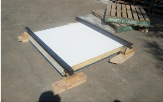
Once again loaded and measured to ascertain the maximum load capacity. It is required that Wind uplift mass should be at least equal the UDL.
