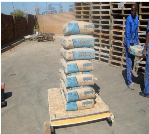
*The deflection measured over the 1200mm length was 4mm with a 650kg load. Afterwards the load was removed and the board went back to normal.*
