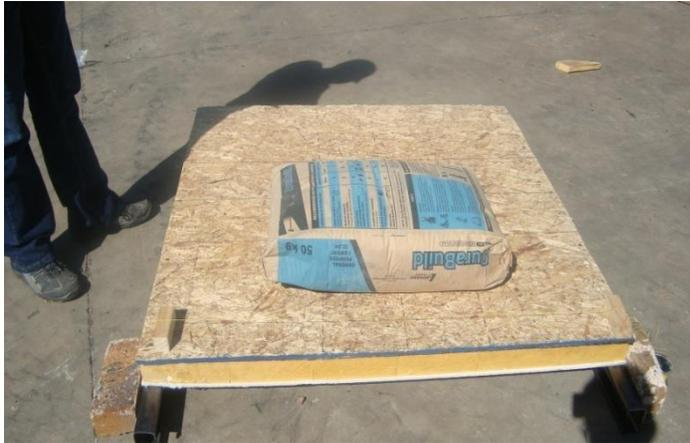
Deflection of the SIPS panels were measured during the investigation with a measuring tape after each 100kg were loaded. The test installation was exposed to increments of 50 kg bags of cement loaded onto the panel by hand. Deflection was continuously recorded and observations were noted of the behaviour of the material.
